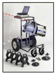
Figure 3 : The ISOCS shield systems and all available components installed on an RDC Ge detector with a Big Mac dewar
