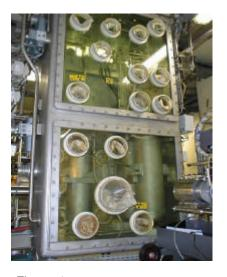
Figure 4 : ISOCS used for in situ spectroscopy in a glove box in a COGEMA facility at Marcoule site
