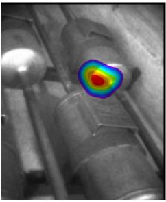
Figure 7 : CARTOGAM view showing a hot spot
