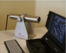
Figure 1 : CARTOGAM detector head, with portable stand and controlling PC
