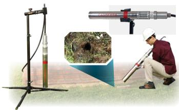
In core spectrometry for Bq/q determination using single sealed LN<sub>2</sub>-free HPGe
