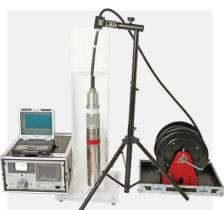
Sealed HPGe in water tank (25 m cable)
