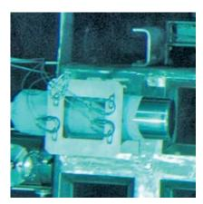
Underwater measurement of activated waste with the **SMOPY Probe**
