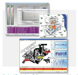
Horizon® Supervisory Software represents a real-time data acquisition and control system that provides supervisory oversight of your radiological instruments. It combines Mirion's radiological monitoring expertise with industry-leading technology for SCADA (Supervisory Control and Data Acquisition) applications.
