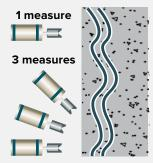
Wall or surface determination in Bg/cm<sup>2</sup> and in-depth profile detection using ISOCS HPGe
