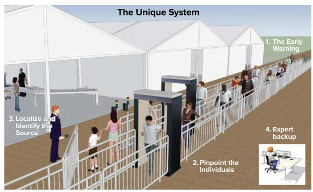
Figure 8. Schematics of arrangement to guide visitors include radiation scan by the FastTrack-Fibre monitor
