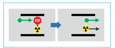
Figure 4. Source taken away from inside the monitor
