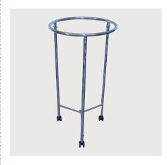
Constructed of stainless steel, this mobile hamper is both durable and clean in its design. All welding accomplished by heliarc method for strength. Exposed welds have been ground smooth to prevent snags.
