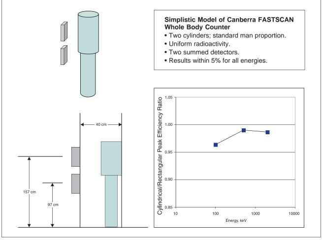
Figure 4. Simulation of the FASTSCAN Whole Body Counter.
