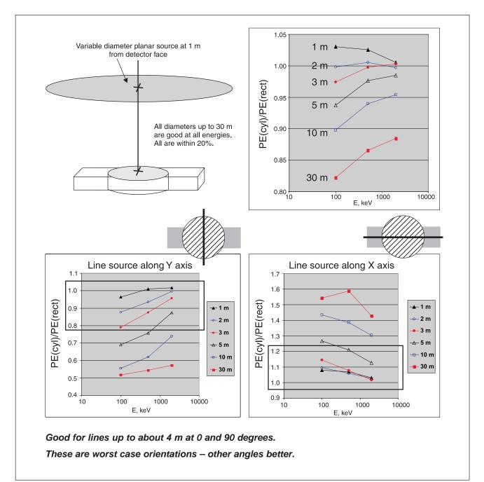
Figure 3. Geometry and results for circular planar source (upper portion) and for linear source (lower portion).
