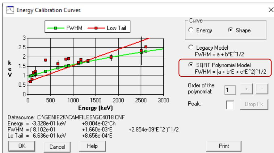
Figure 7 The Energy calibration dialog in Genie. The square root polynomial model selection is highlighted in red.
