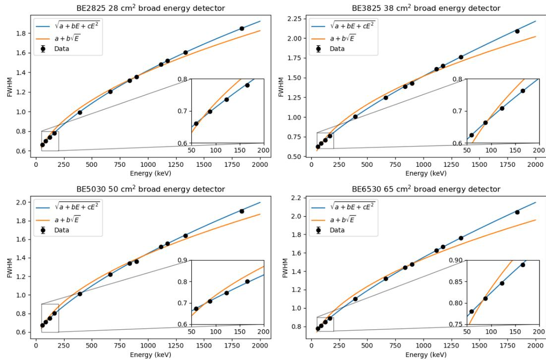
Figure 3 The performance of the new Square Root of Polynomial function and the legacy fit function compared to measured FWHMs and the legacy fit function for different size point contact planar detectors.
