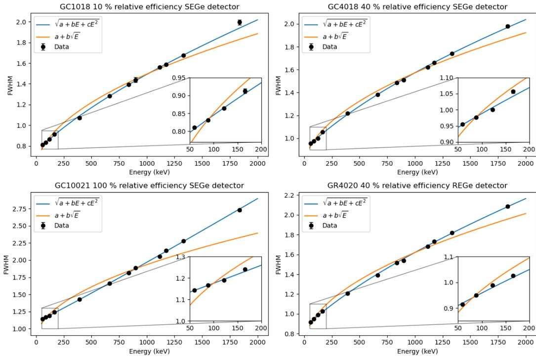
Figure 2 The performance of the new Square Root of Polynomial function and legacy fit function compared to measured FWHM values for SEGe and REGe-type detectors of different relative efficiencies.
