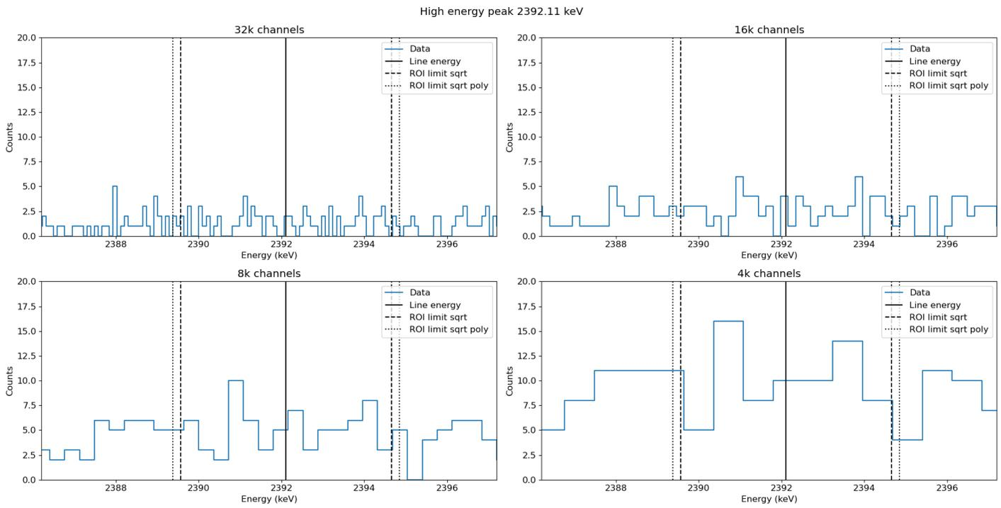
**Figure 5** Examples of the background ROI used to calculate MDA for a high energy emission line for various number of channels in the spectrum.
