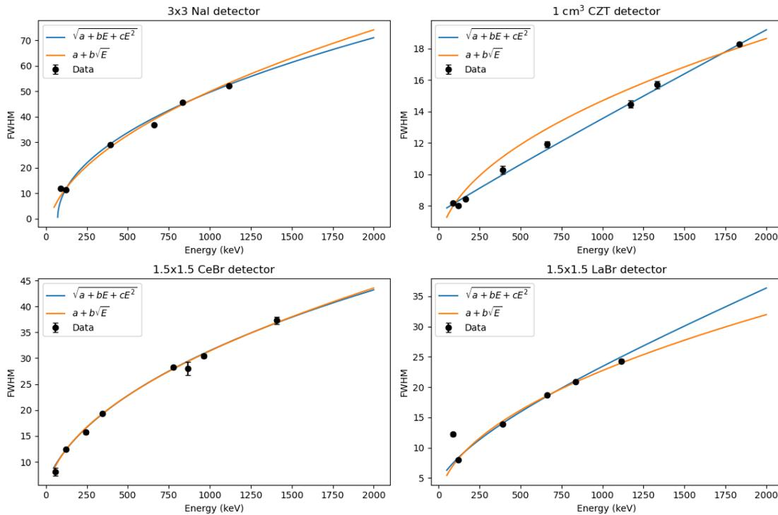
**Figure 4** The performance of the new Square Root of Polynomial function and the legacy fit function compared to measured FWHM values for three types of scintillator detectors and a cadmium zinc telluride (CZT) detector.
