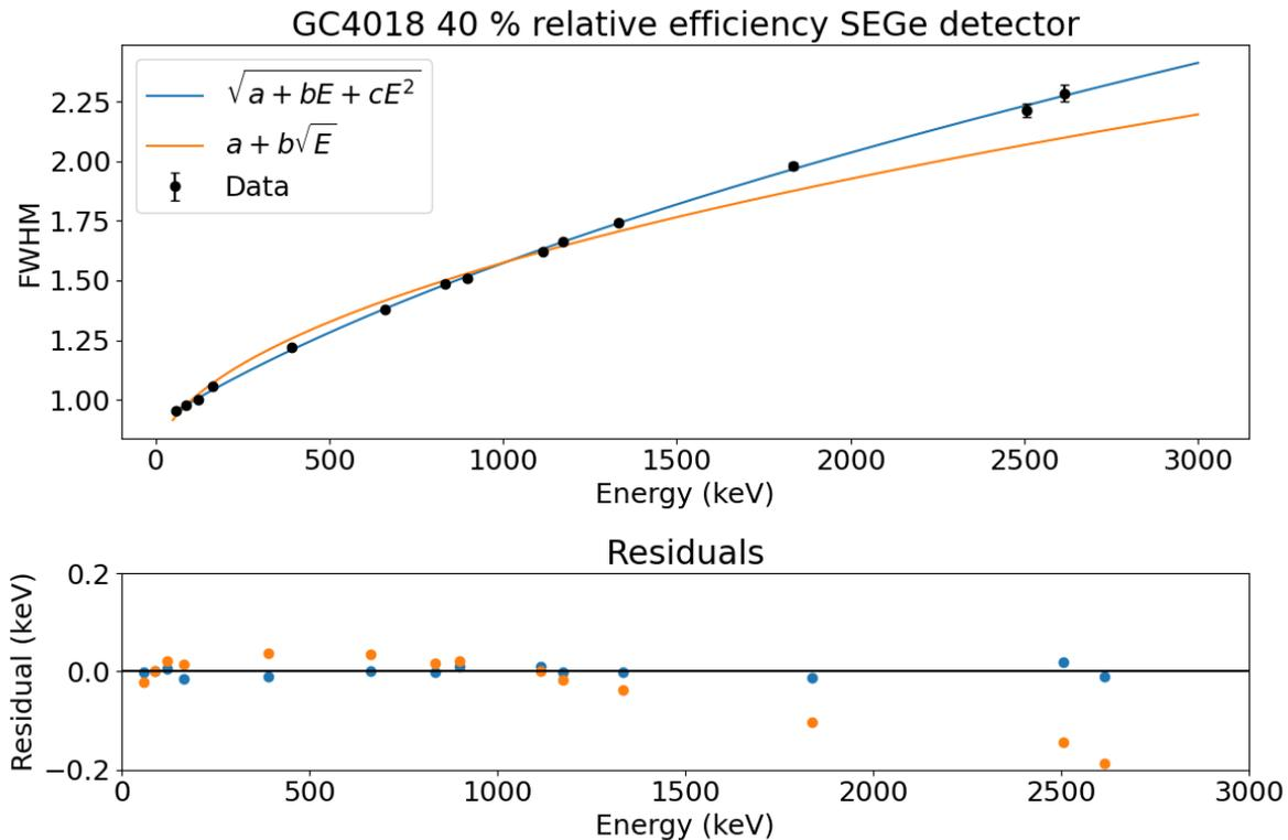
**Figure 1** The performance of the new fit function compared to the legacy fit function for a P-type 40 % relative efficiency HPGe (GC4018) detector. The top figure shows the two fits as a function of energy together with the measured FWHM values. The bottom figure shows the residuals between the fits and the measured FWHM values.
