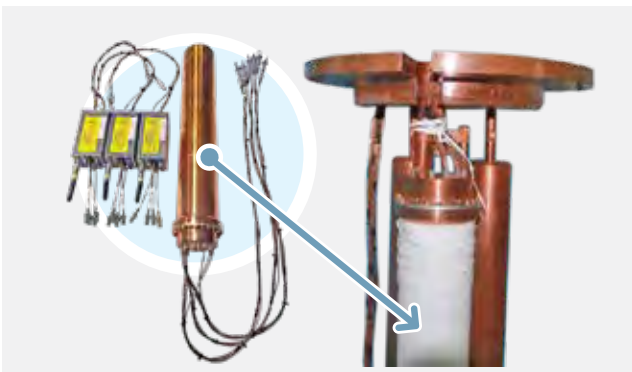
Array detector with three PCGe detectors to be dipped in LAr
