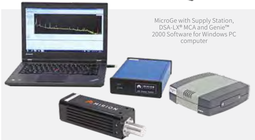
A novel, ultra-compact, gamma spectroscopy detector for high count rates in confined spaces.
