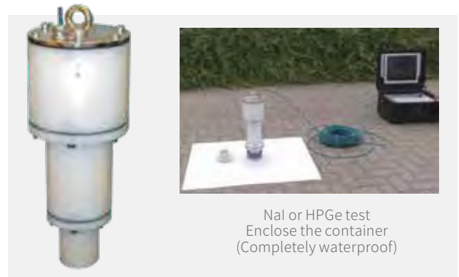
Sealed HPGe Probe for LN 2 -free operation in harsh environments
