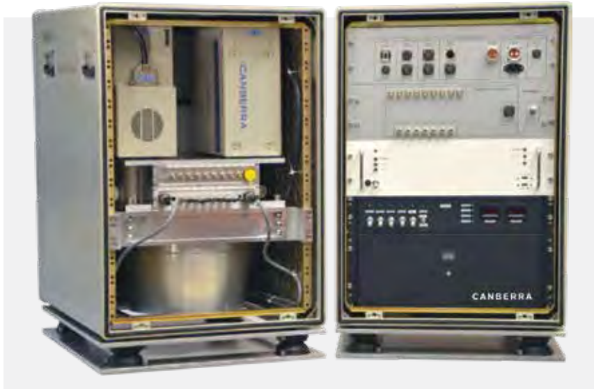
Hardware overview of the Mirion airborne system consisting of two cabinets (detector and processing electronics)
