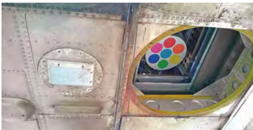
View of detector cap through a hole in aircraft cabin. Each colored circle shows the location of an individual coaxial detector within a common cryostat
