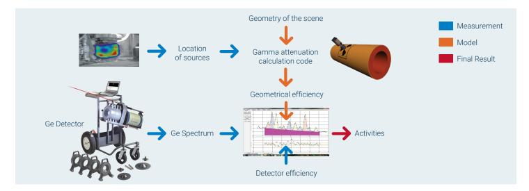
ISOCS Uncertainties Estimator and multi-Geometry Calculator enables the testing of the sensitivity of model's parameters, such as geometry, material, shapes, etc.
