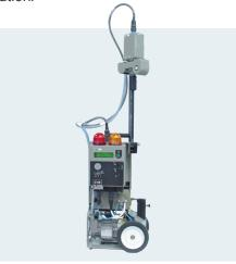
ABPM 203M<sup>™</sup> Mobile Alpha/Beta Particulate Monitor. This monitor, with its small and lightweight extendable sensor, functions locally next to the respiratory tract of workers. It is perfectly adapted for the measurement of particulates in environments with high rates of radon.
