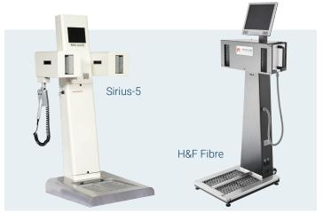
Sirius<sup>™</sup>-5 (gas or gasless) and H&F Fibre (gasless) for  $\alpha\text{-}\beta$  contamination monitoring purposes
