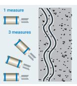
Wall or surface determination in Bq/cm<sup>2</sup> and in-depth profile detection using ISOCS HPGe
