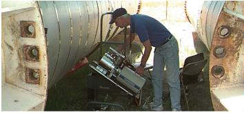
Flexible geometrical models for efficiency determination using ISOCS software
