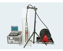
Sealed HPGe in water tank (25 m cable)
