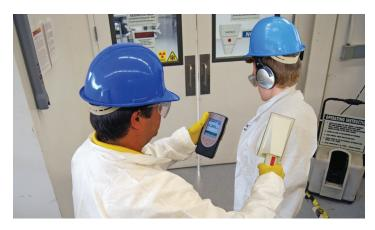
The Radiagem and Colibri family can accommodate a family of CSP-Smart probes for enhanced detection of gamma dose rate and  $\alpha$ - $\beta$  ( $\gamma$ ) contamination monitoring
