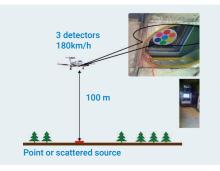
Air survey mapping with segmented HPGe detectors
