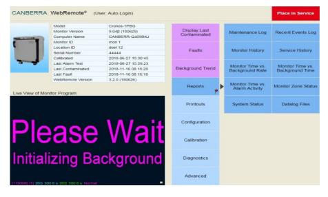
The monitor will also take itself out of service if the calibration interval is exceeded or other operational conditions exist, which prevents the unit from achieving the desired sensitivity. These conditions can be configured by the user. Calibration can be easily executed by just one person and is highly automated.
