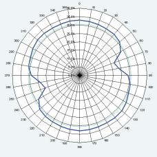
Argos-5AB Horizontal Scan Efficiency for <sup>36</sup>Cl, Phantom 5 cm from Center Detector.
