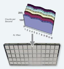
This diagram shows the counts detected by placing a button source in 60 different positions along and across the detector. The uniformity of response is remarkable (±8%). The huge degradation (±50%) exhibited by some of the Mirion competitors, particularly in the corners, has been significantly minimized.
