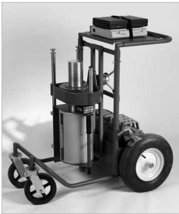
Figure 10 ISOCS shield ready to move to new location; all shield accessories fit into carrying tray on back; computer and MCA can be strapped down to tray on top.
