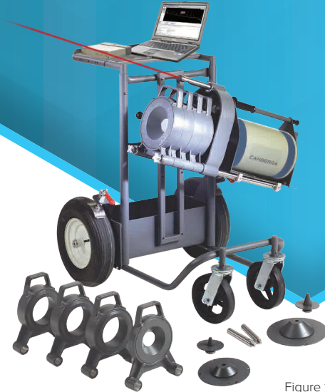
Figure 1 The ISOCS Shield Systems and all of their available components installed on an RDC Ge Detector with a Big MAC Dewar. (See Figure 3 for more details.)
