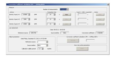
A Wizard settings adjustment module helps to adapt CSPS software to existing calibration source of most available radioisotopes and to define the expected calibration result, ensuring all users will follow the same easy to go procedure. Each calibration step parameter is available and can be tuned to offer a turnkey calibration matching major site expectations and procedure.
