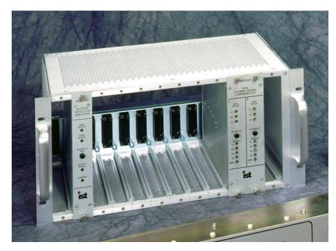
The NPB-2004 (shown with optional NPA-2002 and NPC-2003 NIMs installed) Houses and provides power to Nuclear Instrumentation Modules (NIMs)
