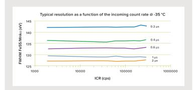
Figure 3 - Typical resolution as a function of the incoming count rate for different peaking times (using a flat top of 0.1  $\mu s$  and at -35 °C).
