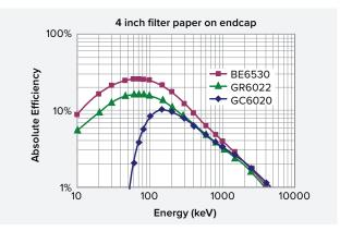
Absolute Efficiency vs. Energy Comparison for BE6530, GR6022 (n-type coaxial) and GC6020 (p-type coaxial) detectors – all with 60% Relative Efficiency @ 1332 keV
