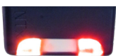
Red flashes of the left and right LED: eTx Module in alarm
