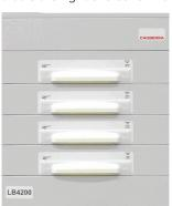
The LB4200 counter can be equipped one to four drawers. Each counting drawer contains high quality gas-flow pancake style proportional detectors with ultra thin low background windows to provide the greatest measurement sensitivity. Drawers can be upgraded individually and are completely self-contained; no controller upgrades are necessary to add a drawer.
