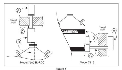
Cryostat designs suitable for low-background detector systems
