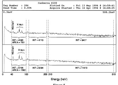
Figure 5 Background spectra from lead samples Top -  $^{210}$ Pb content  $\approx$  20 mBq/gm Bottom -  $^{210}$ Pb content  $\approx$  60 mBq/gm
