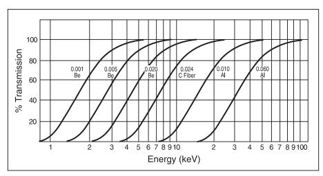
Figure 3 Window transmission characteristics
