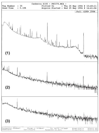
Figure 8 Background from 40% coaxial detector (1) unshielded (2) shielded with standard cryostat and (3) shielded with Ultra Low-background cryostat
