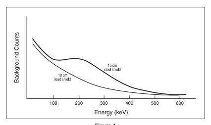
Figure 4 Background continuum vs shield material
