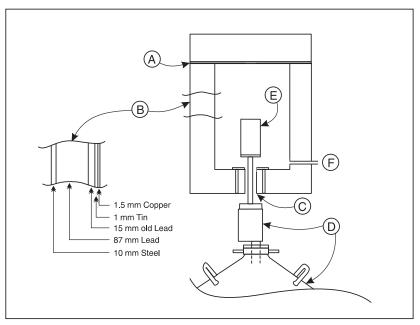
Figure 7 Ultra low-background shield design and cross-section of materials
