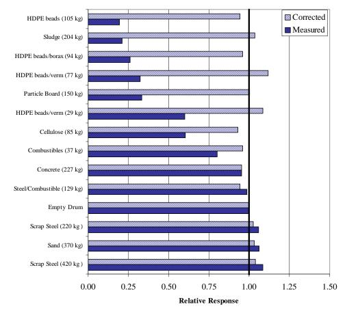
Figure 3. Measured performance of the Add-A-Source correction technique for uniform source and matrix distributions. The solid bars show the relative performance prior to application of the AAS correction.
