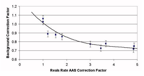
Figure 4. Plot of the neutron coincidence background as a function of AAS correction factor for the drum. The data points show the observed reduction in the empty chamber coincidence rate for a series of drums with increasing moderator content.
