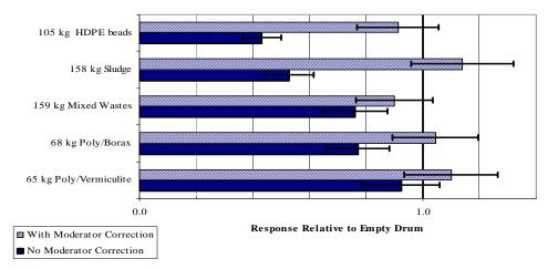
Figure 7. Relative performance of the active neutron matrix correction using the AAS based moderator index for an HEU point source. The results displayed relative to the effective uranium mass (0.28 grams  $^{235}$ U).
