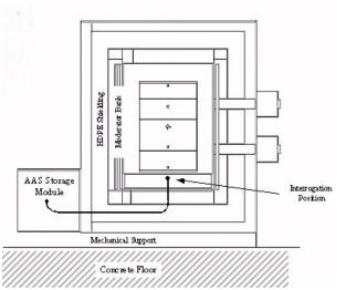
Figure 2. Sketch of the layout of the IWAS assay cavity. The figure shows the AAS source interrogation position in the center of the rotator assembly below the center of the drum.
