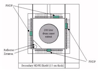
Figure 5. Sketch of the layout of the IWAS active neutron subsystem. The figure shows the location of the four fast Cd covered neutron detection packages (FNDP).
