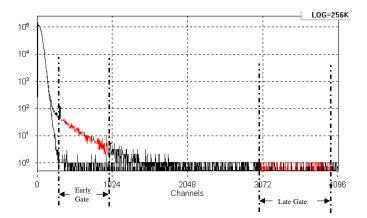
Figure 6. Time response of the Fast Neutron Detector Packages for a zero matrix drum. The upper curve shows the response for a 1 gram  $^{235}$ U source and the lower for a drum with no fissile material. (The time scale is 2 µsec per channel).
